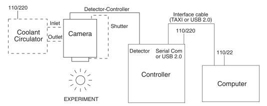
Figure 7. System Connection Diagram (TE Camera)
